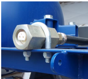
Figure 20: Ensure EOC Receptacle is Free of Debris
