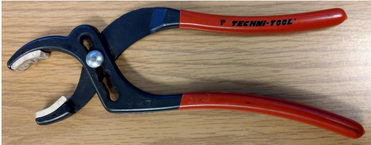
Figure 18: Soft Jaw Pliers Used to Prevent Cable Twisting When Turning the Hexnut
